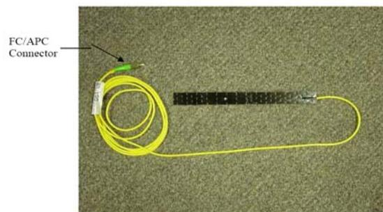
Figure 2 Composite deck mountable packaged sensor
