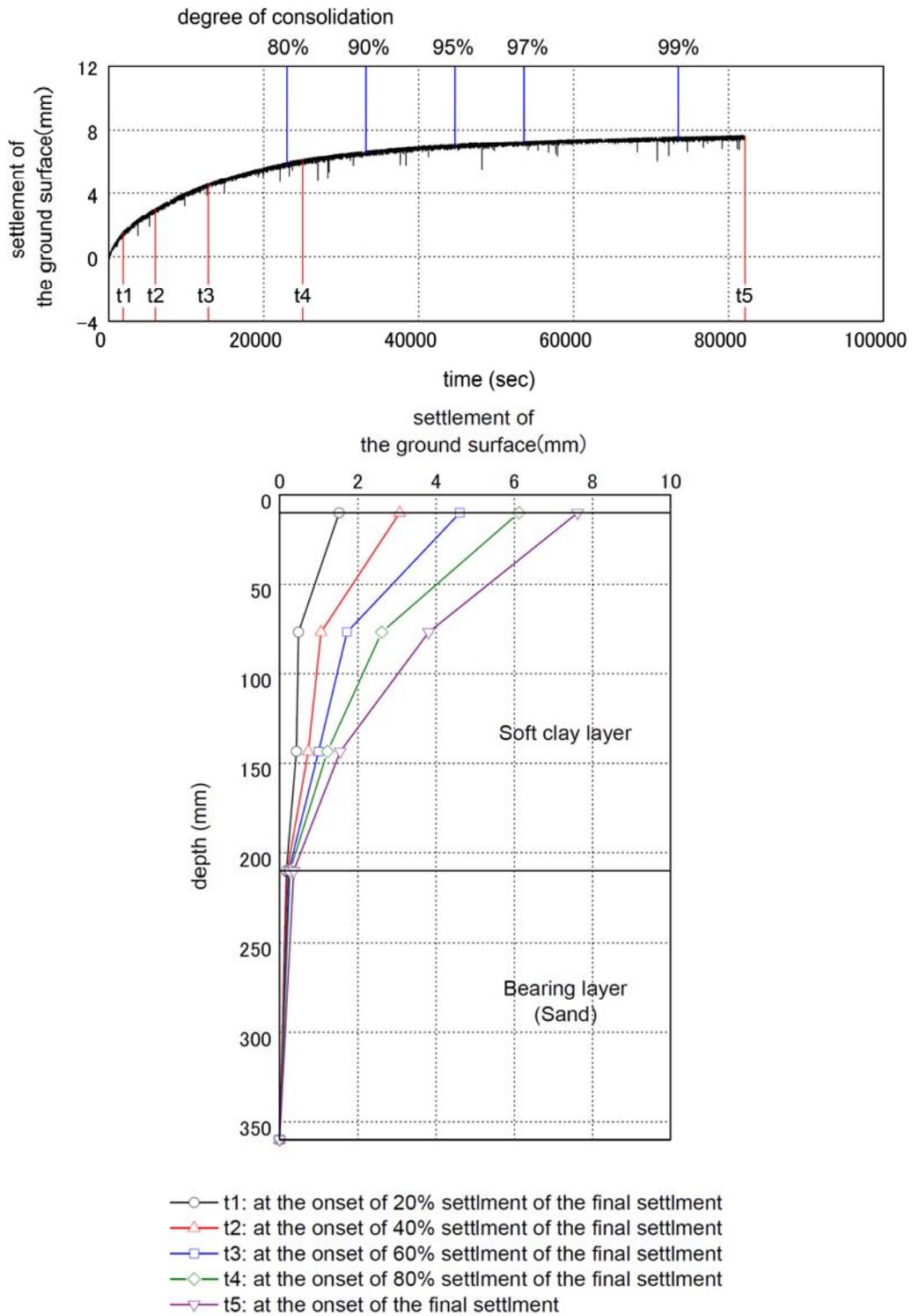
Fig. 3 Histories of the settlement of the soft clay layer's surface and the distribution in the depth direction
