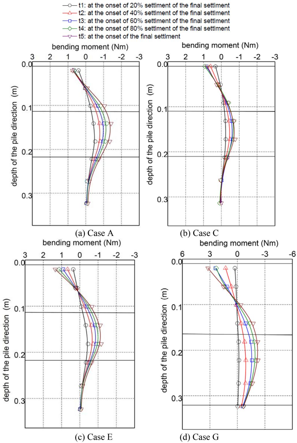
Fig. 4 Distribution of the bending moment(experimental data)
