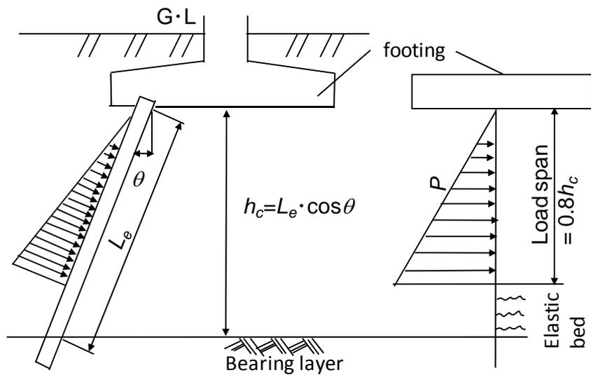
Fig. 1 Conceptual diagram of Sato's equation
