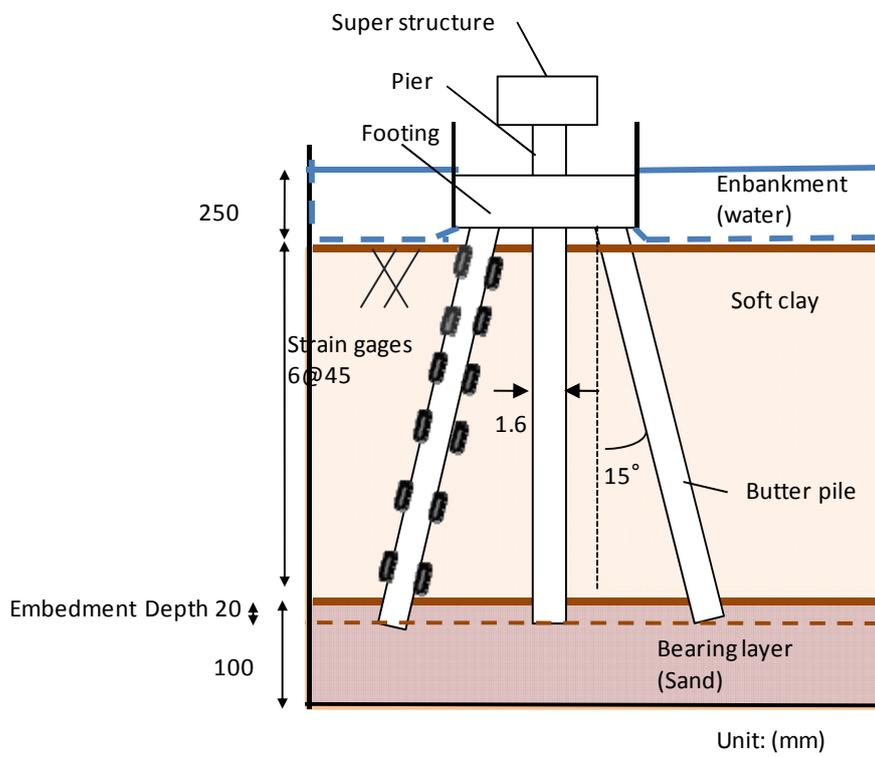
Fig. 2 Experimental setup for consolidated load centrifuge experiment
