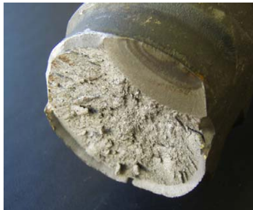
FIGURE 8-CLOSE-UP OF FRACTURE HS ROD.
