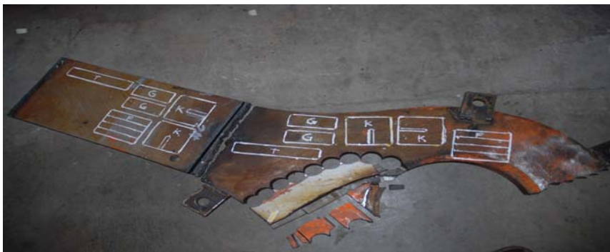
FIGURE 6-DETAILED TESTS WERE PERFORMED ON THE STEEL FROM THE CRACKED EYE BAR.
