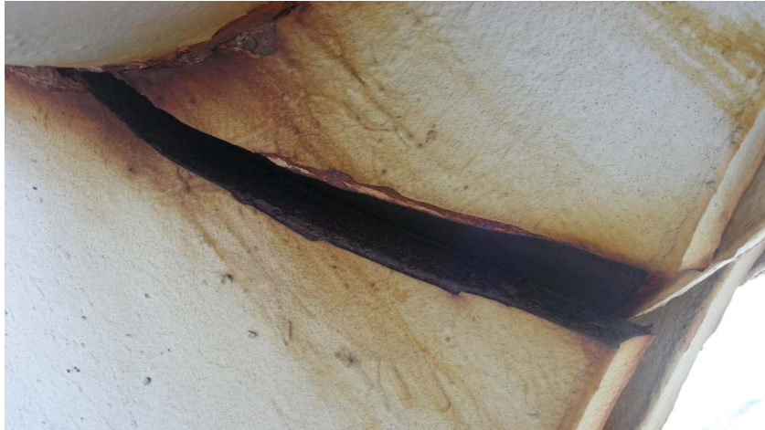
FIGURE 1-THE FRACTURE PROPAGATED ACROSS THE FULL WIDTH OF ONE SIDE OF THE EYE SECTION OF THE EYE BAR.
