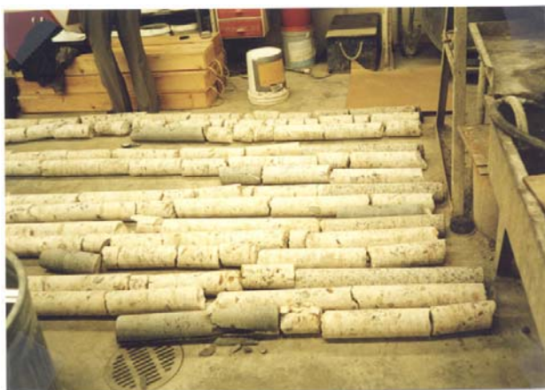
Figure 4. Vertical cores during inspection in the PANYNJ materials laboratory
