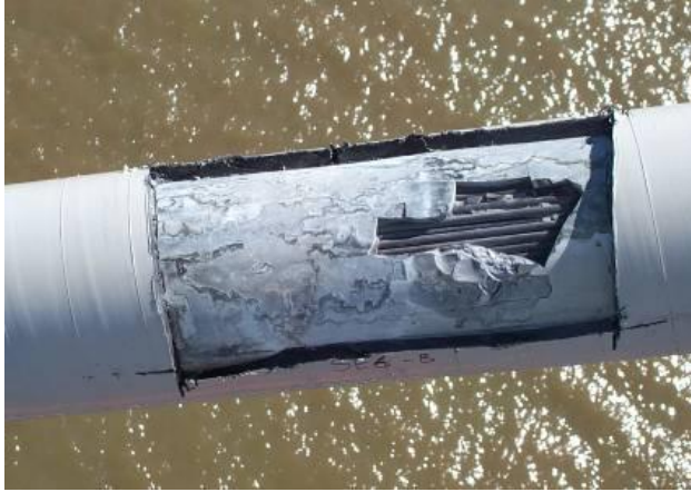
FIGURE 2- DISSECTION OF EXISTING CABLE
