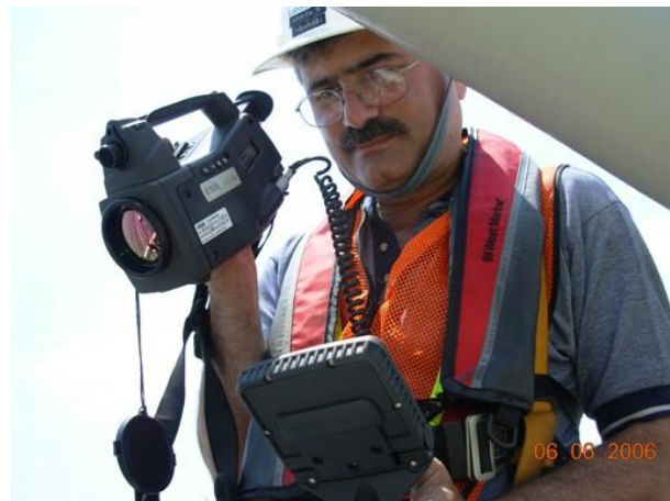
FIGURE 5- NDT USING THERMOGRAPHY
