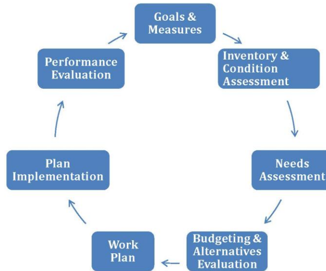
FIGURE 3, THE SYSTEMATIC PREVENTIVE MAINTENANCE PROCESS 5
