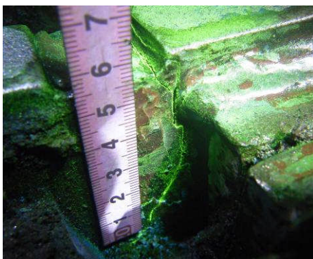
Fig.11 Cracks penetrated to base metal
