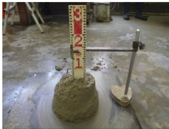
Fig.6 The condition of FACET in accordance with slump test (JIS A 1101)
