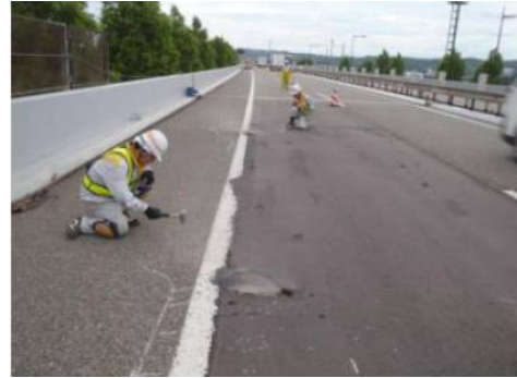
Fig.3 The delaminated RC decks caused by deicing Fig.4 Typical investigation of RC decks
