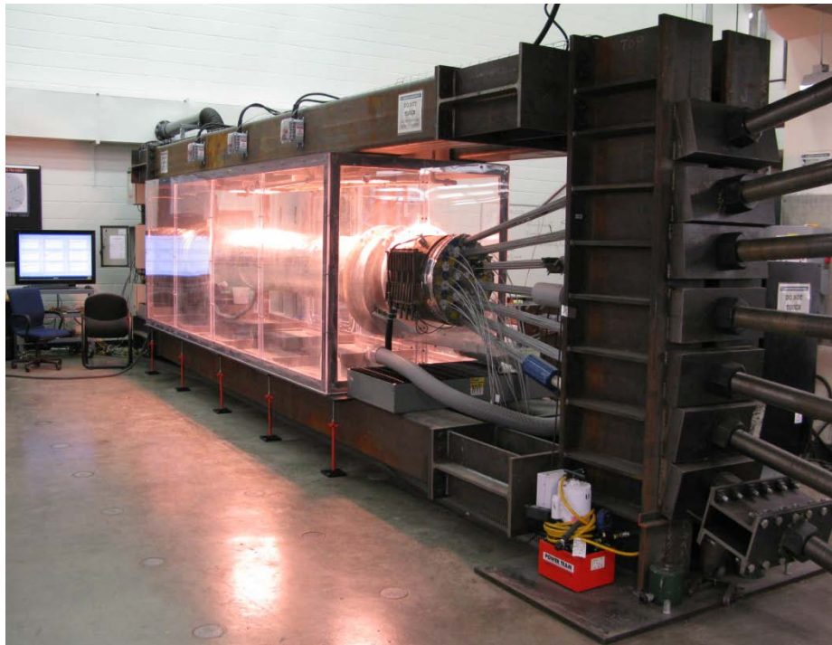
Figure 3: Cable mock up and environmental chamber
