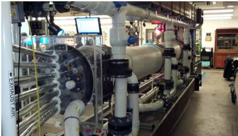
Figure 6: Front and Back View of the Cable Mock-up with Dehumidification System
