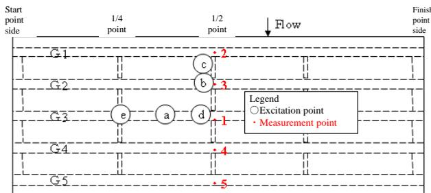
Figure 11. Excitation point and the measurement point
