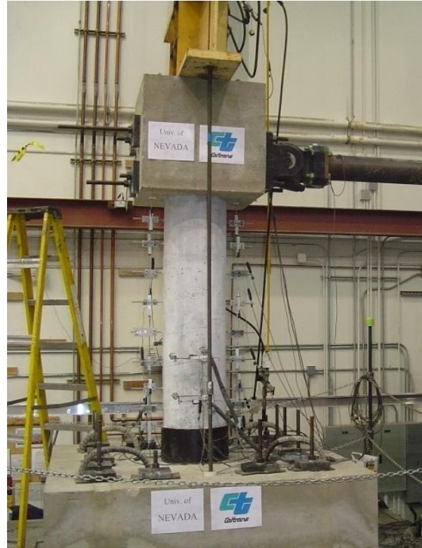
Fig.11 – Segmental column model with rubber pad a shake table at the University of Nevada - Reno
