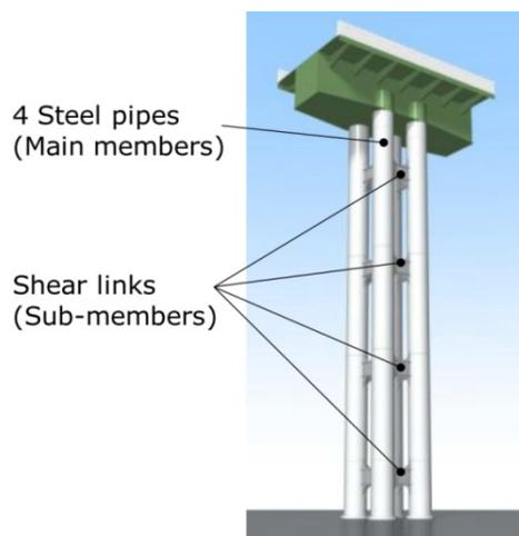
**Fig-1 Steel pipe integrated pier**
