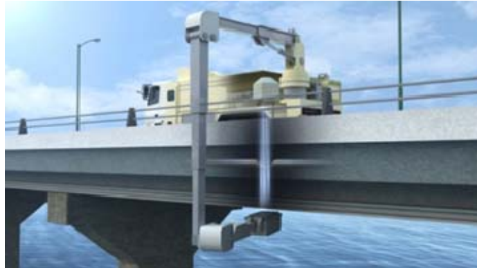
Figure 16 image of portable neutron imaging device (source: RIKEN)
