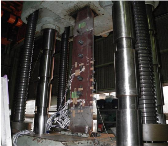
Photo 6 Static tensile test of single-spliced bolted adhesive joints<sup>6)</sup>
