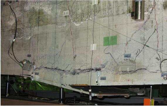
Photo 4 Debonding failure of splice plates on specimen S1
