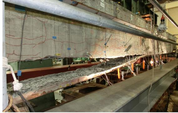
Photo 5 Debonding failure from ends of steel plate (near side in the photo) of specimen S4 (immediately after maximum load is applied)
