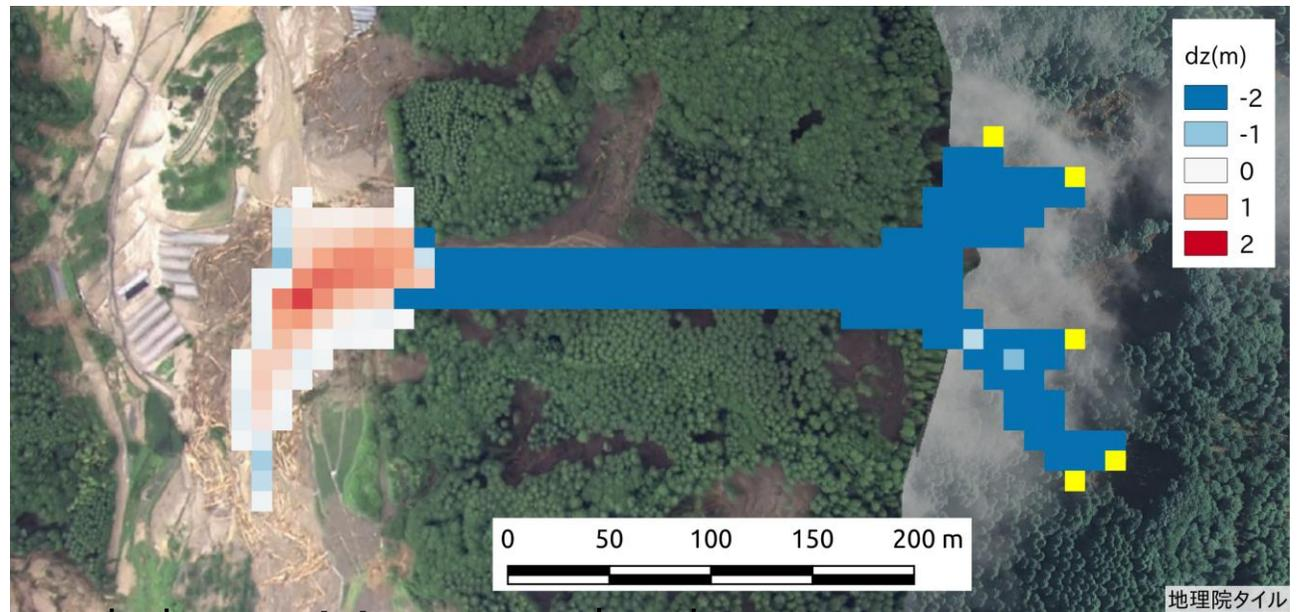
Spatial distribution for erosion and deposition resulted from debris flow
