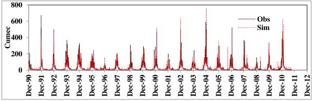
Figure 6: Model simulation and ground observed runoff at Rugam
