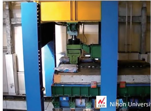
Wheel loading test of RC slab specimen
