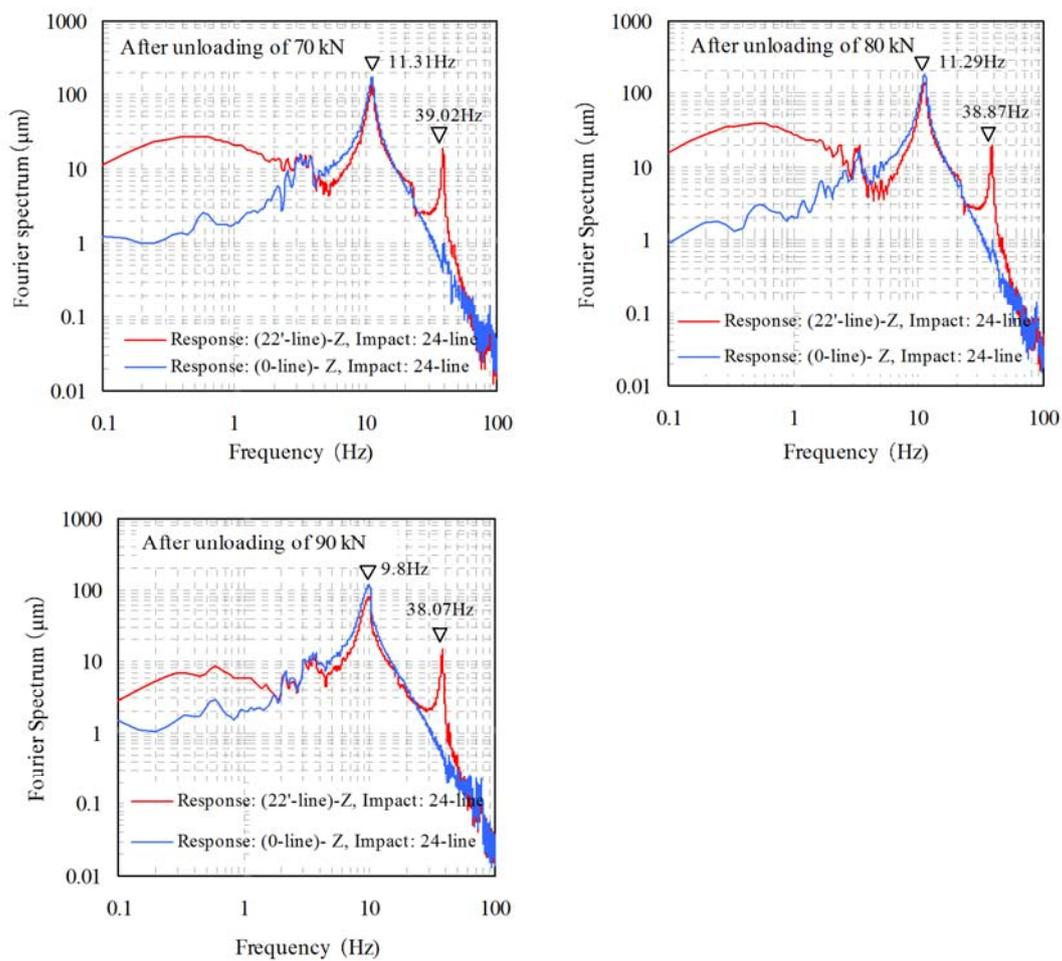
Analysis were done after unloading of each cycle, Sampling frequency:200 Hz, Bandwidth: 0.2 Hz.
