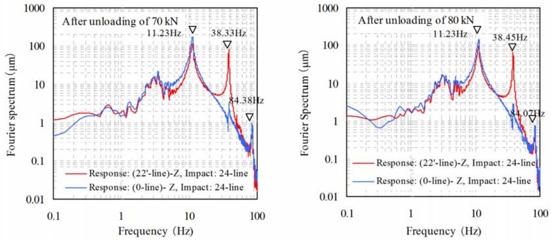
Analysis were done after unloading of each cycle, Sampling frequency:200 Hz, Bandwidth: 0.2 Hz.
