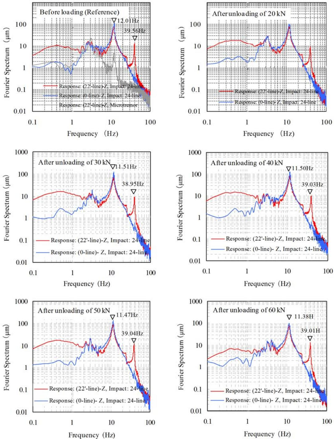
Analysis were done after unloading of each cycle, Sampling frequency:200 Hz, Bandwidth: 0.2 Hz.
