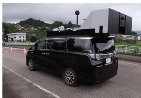
写真 1-3-7 MMS (Mobile Mapping System)
