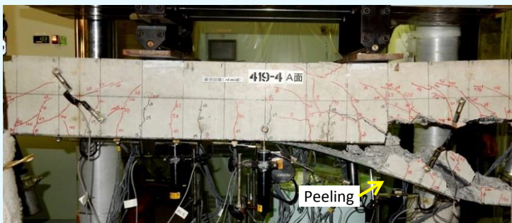
Sheet peeling in a flexural test
