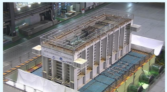
Experiment using E-Defense to develop earthquake-resistant reinforcement technology for bridges on liquefied soil
