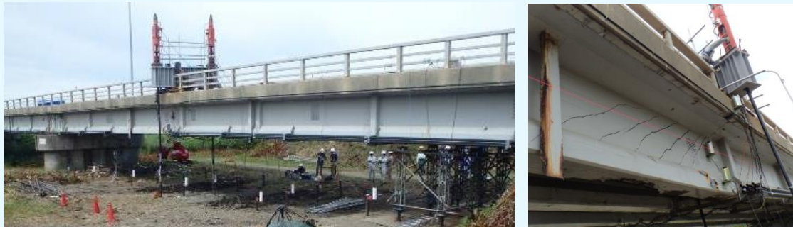
On-site loading test on a bridge to be removed, until it collapses
