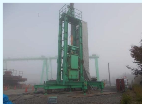
Rapid loading test (with an actual pile) being conducted
