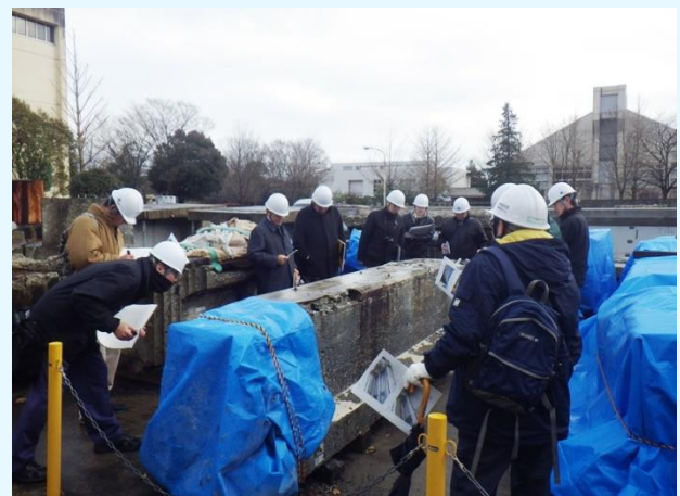
Examination practice at an exhibition facility of removed members (Carried out as part of the training of the College of Land, Infrastructure, Transport and Tourism. The case is studied with a deteriorated member who has been removed)
