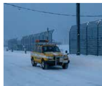
Measuring the effectiveness of snow fences using a mobile observation vehicle with impaired visibility to develop a method for evaluating the performance of snow fences
