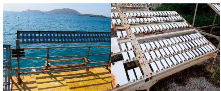
Verification of durability of highly weather-resistant paints and corrosion-resistant metal via exposure testing
