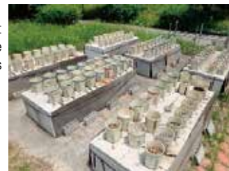
◀ Experimental reinforced soil wall (8 m height) for long-term observation
