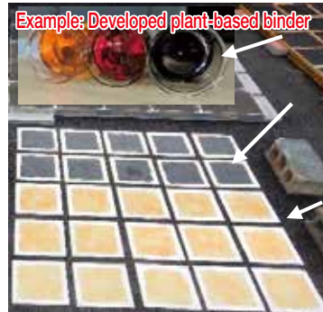
Development of paving materials using plant-based binders (photo:outdoor exposure testing for weather resistance)
