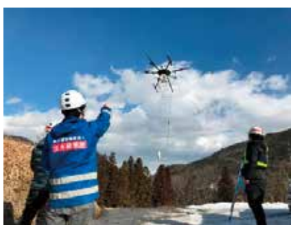
UAV electromagnetic survey at the Komatsubara Landslide, Nagano City
