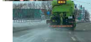
Development and testing of an antifreeze spraying support system, with the aim of operation by a single driver
