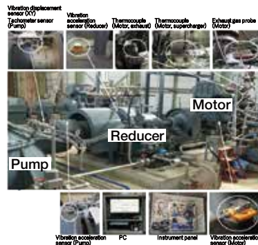
Pump equipment condition monitoring system
