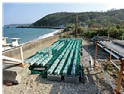
Outdoor exposure tests of concrete specimens
