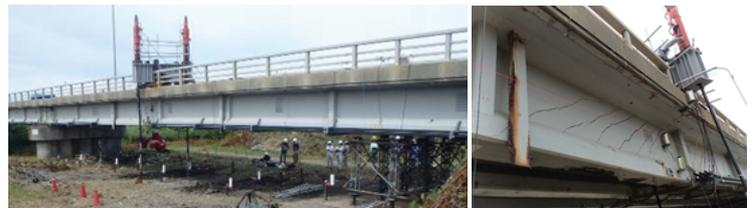
Failure testing of PC main girders of actual bridges for the first time in Japan to develop a load-bearing capacity assessment method
