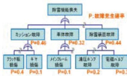
Analysis of probable failure of snow removal machines using FTA
