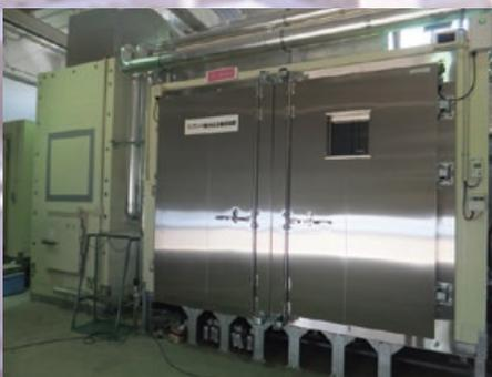
Concrete combined-deterioration accelerating test apparatus
