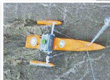
Flow rate observation technology using the ADCP
