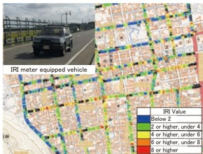
Studying methods of easily identifying pavement that requires maintenance (Use of IRI values)(pavement)
