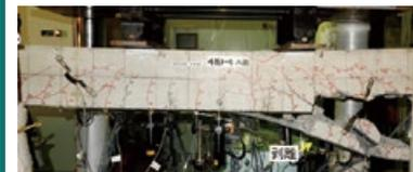
Beam Test is performed to propose a design method for retrofitting using fiber sheets (bridges)
