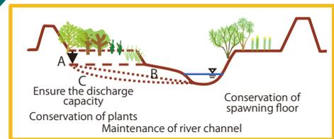
Not only ensure the discharge capacity but also develop river channel excavation technology to contribute to conservation and restoration of the diversity of plants, good fish habitat/spawning environment in the land. Also develop technology for subsequent maintenance methods.
