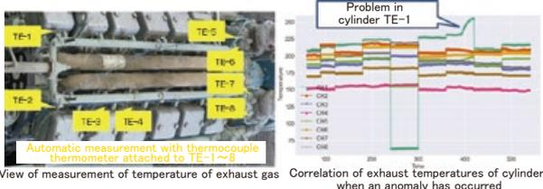
View of measurement of temperature of exhaust gas
