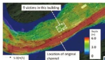
Results of the analysis of flood discharge after change in the riverbed and flow channel of a valley floor river in a semi-mountainous area
