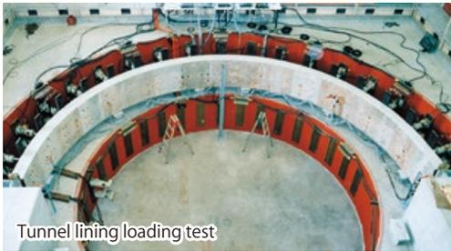
Tunnel lining loading test
