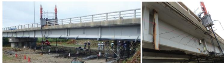
Failure testing of PC main girders of actual bridges for the first time in Japan to develop a load-bearing capacity assessment method
