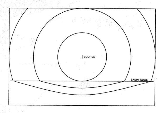
Figure 1. Schematic plan view of the wavefronts for an S wave from a point source converting to a surface wave at the edge of a basin. The phase velocity of the surface wave is one-third the S wave velocity.
