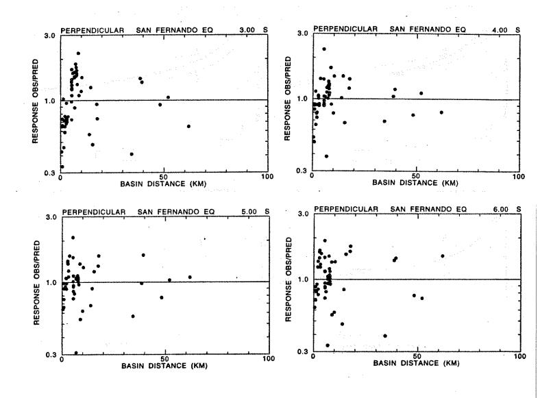
Figure 7. Ratios between observed values of pseudovelocity response and values predicted by equation (1) for the perpendicular component of the San Fernando earthquake.
