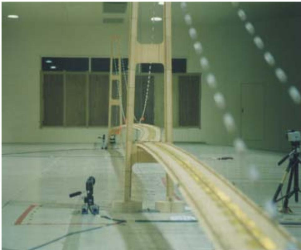
Photo 1 Static deformation of super long-span bridge (wind speed=8m/s)
