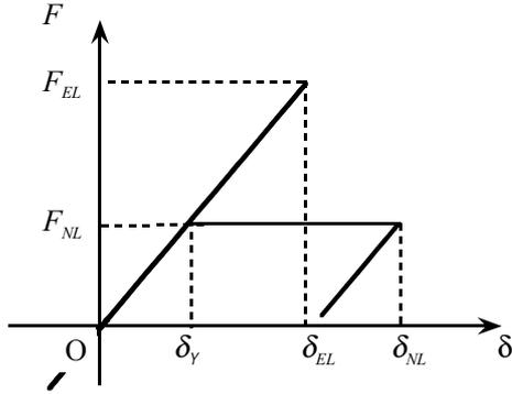
Fig. 1 Definition of Force reduction Factor
