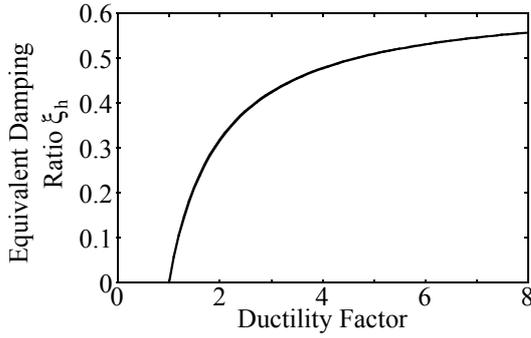
Fig.2 Equivalent Damping Ratio  $\xi_h$  by Eq. (4)
