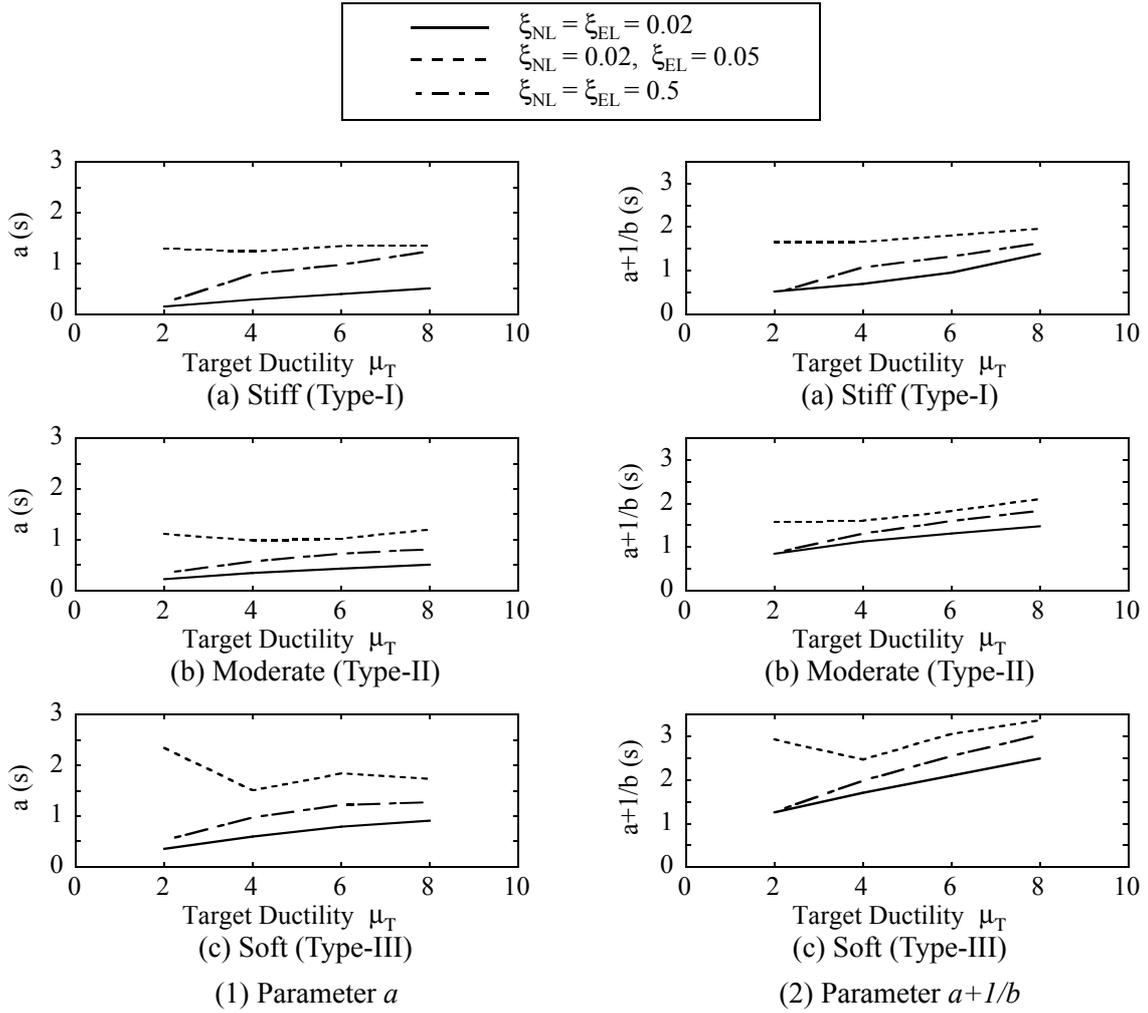
Fig. 14 Dependence of Parameters  $a$  and  $a+1/b$  on the Assumption of Damping Ratios
