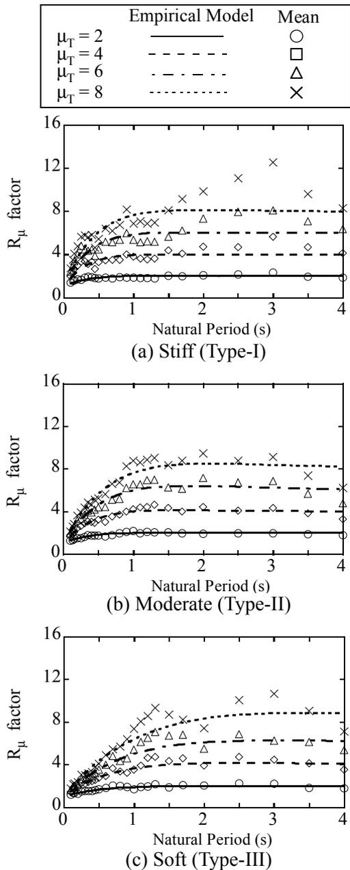
Fig. 11 Application of Eq. (19) to the Mean Force Reduction Factors Presented in Fig. 5
