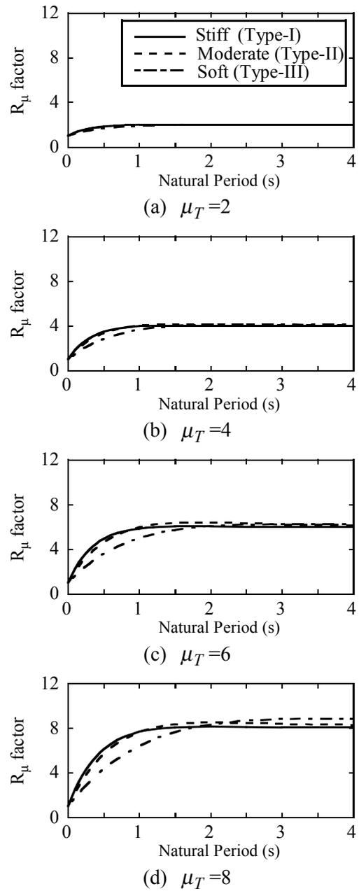
Fig. 12 Effect of Soil Condition on the Force Reduction Factors Predicted by Eq. (19)
