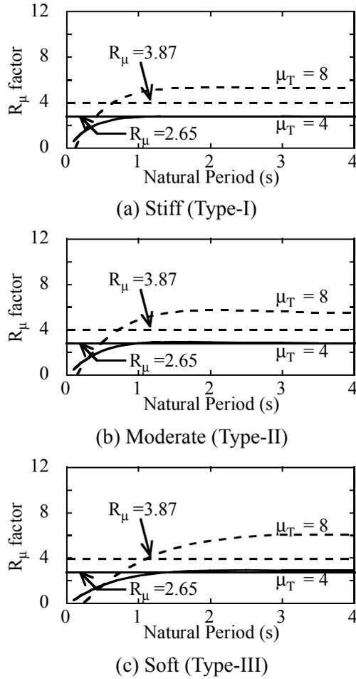
Fig.13 Force Reduction Factors Corresponding to Means minus One Standard Deviations
