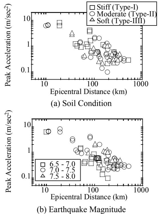
Fig. 3 Classification of Ground Accelerations in Terms of Soil Conditions and Earthquake Magnitudes
