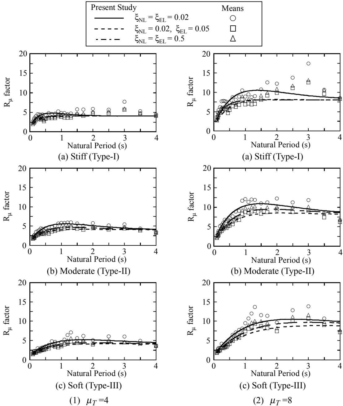
Fig. 15 Dependence of Force Reduction Factors on the Assumption of Damping Ratios
