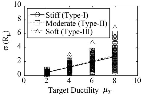
Fig. 7 Target Ductility Factor Dependence of the Standard Deviations of Force reduction Factors
