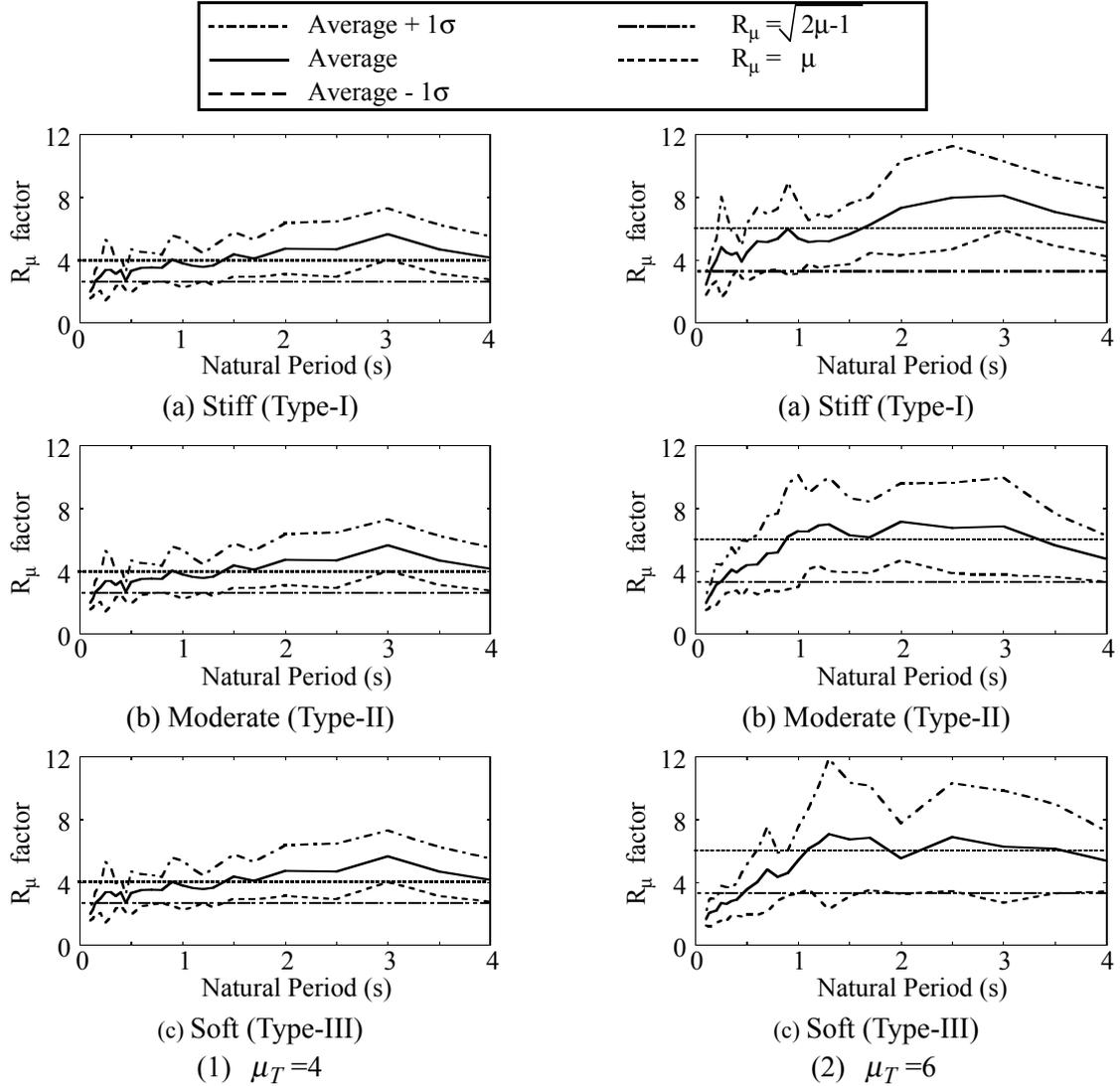
Fig. 5 Mean and Mean +/- One Standard Deviation of the Force Reduction Factors for 70 Ground Motions
