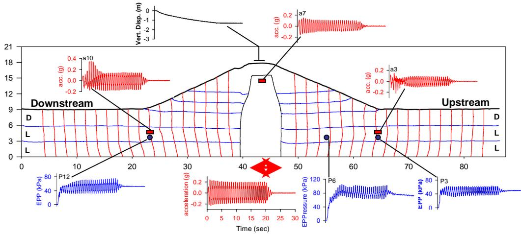
Figure 3. Model 2 selected transducer data and post-shake mid-cross-section.
