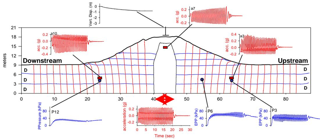
Figure 5. Model 4 selected transducer data and post-shake mid-cross-section.
