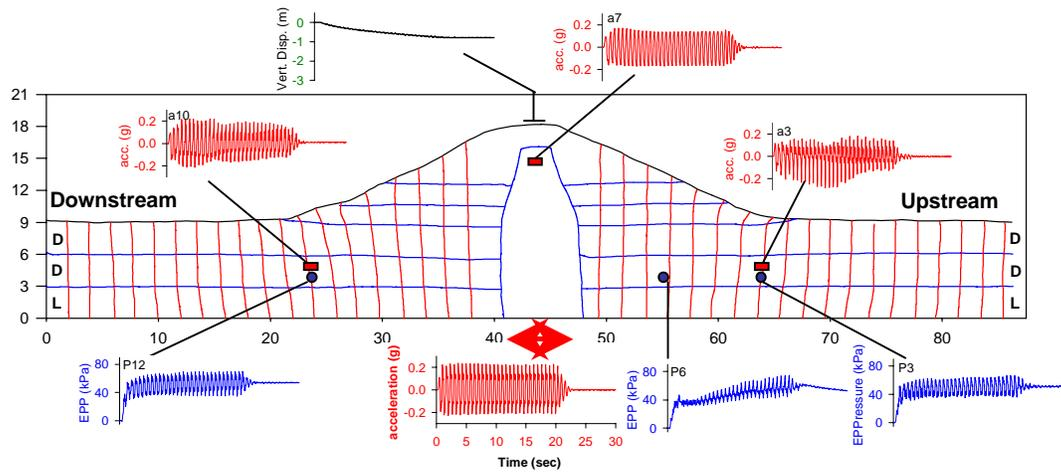
Figure 4. Model 3 selected transducer data and post-shake mid-cross-section.
