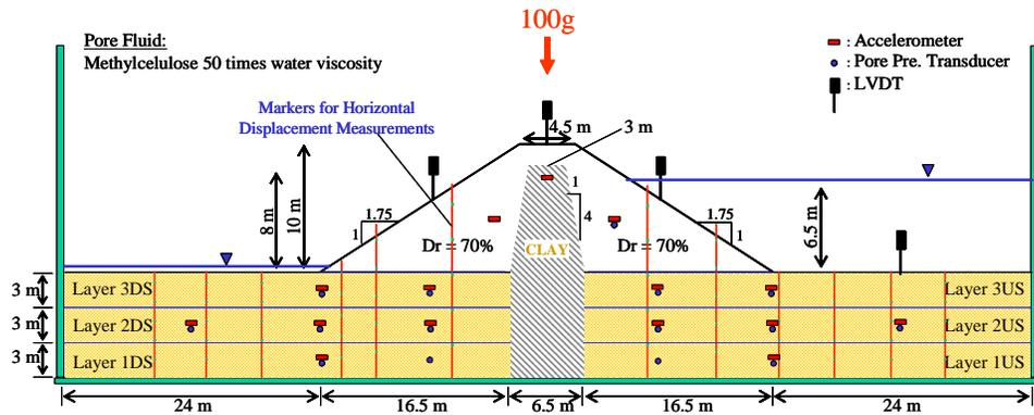
Fig.1 Schematic of a typical dam-foundation model.
