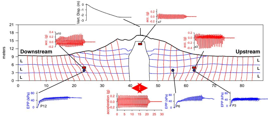
Figure 2. Model 1 selected transducer data and post-shake mid-cross-section.
