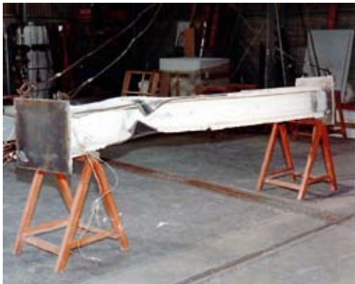
Photo 6. Buckling of Column after Loaded Heat Test
