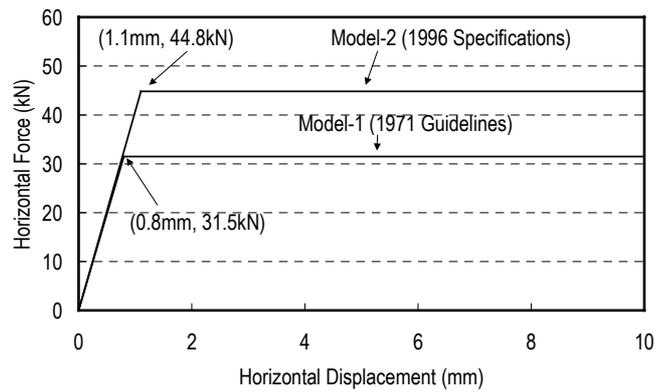
Fig. 7 Horizontal force-displacement relationship of pier
