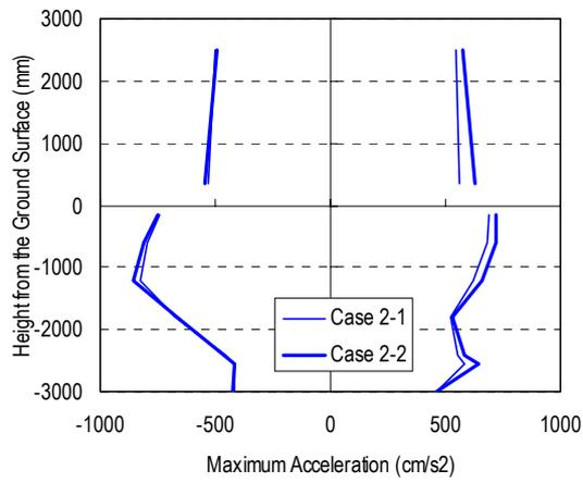
Fig.9 Maximum acceleration distribution (Cases 2-1 and 2-2)
