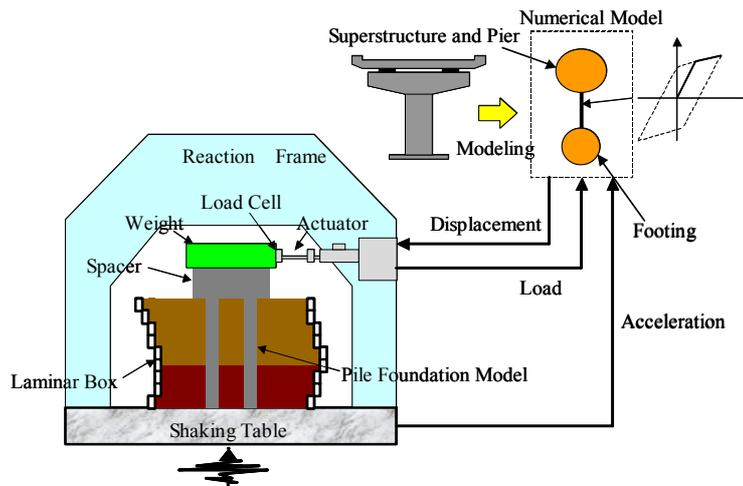
Fig.1 Conceptual view of hybrid vibration experiment
