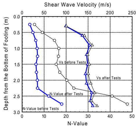
Fig.4 N-value and shear-wave velocity of ground model
