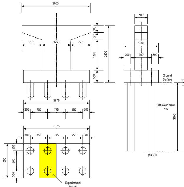
Fig. 6 Overview of experimental model on the liquefiable ground
