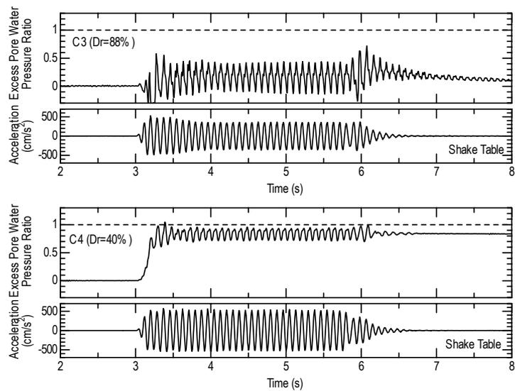
Fig.14 Excess pore water pressure ratio at 0.95m beneath the surface (Cases C3 and C4)
