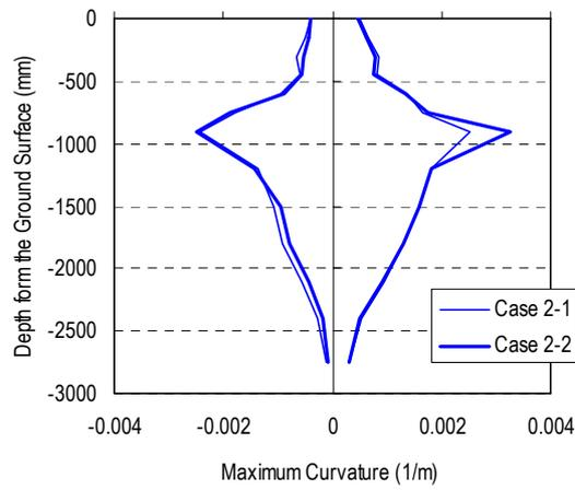
Fig.10 Maximum curvature distribution (Cases 2-1 and 2-2)
