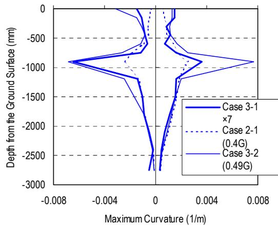
Fig.12 Maximum curvature distribution (Cases 3-1, 2-1 and 3-2)
