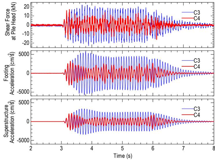
Fig.16 Shear force at pile head, accelerations at footing and superstructure (Cases C3 and C4)
