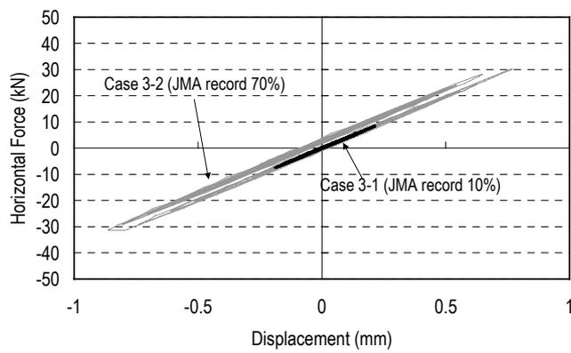
Fig.11 Horizontal force-displacement relationship of pier (Cases 3-1 and 3-2)
