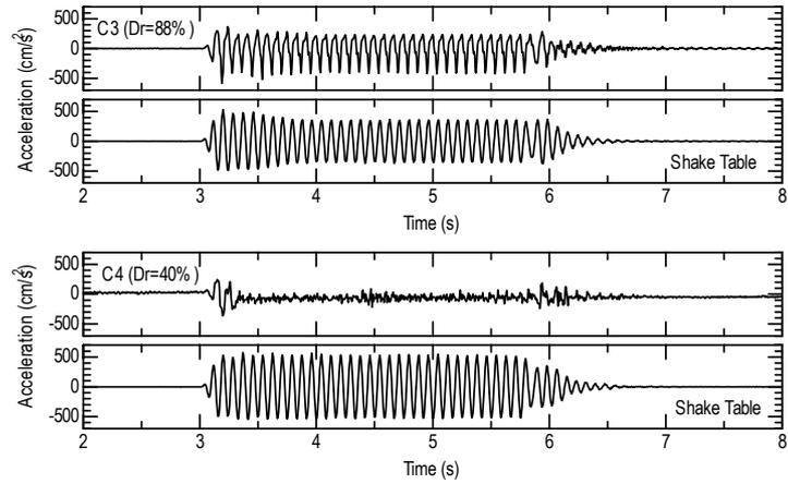
Fig.15 Acceleration at 0.95m beneath the surface (Cases C3 and C4)
