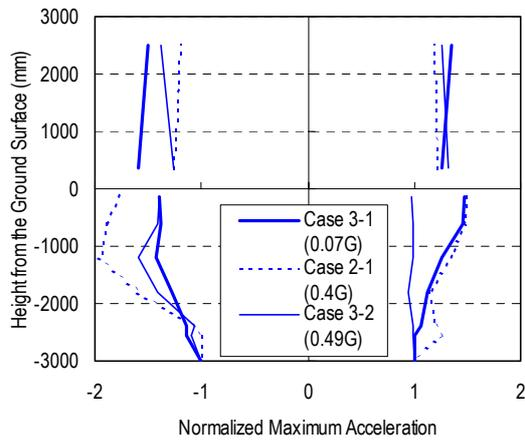
Fig.13 Maximum acceleration distribution (Cases 3-1, 2-1 and 3-2)
