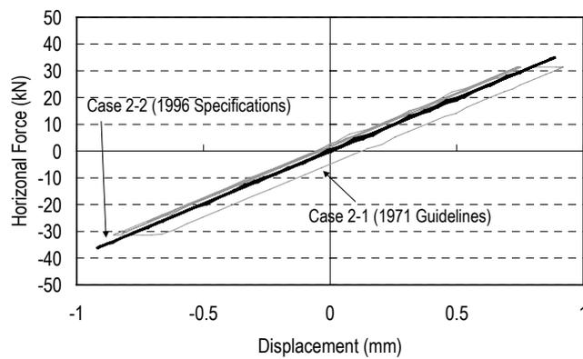
Fig. 8 Horizontal force-displacement relationship of pier (Cases 2-1 and 2-2)
