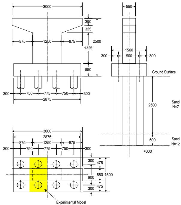
Fig.3 Overview of experimental model on the non-liquefiable ground
