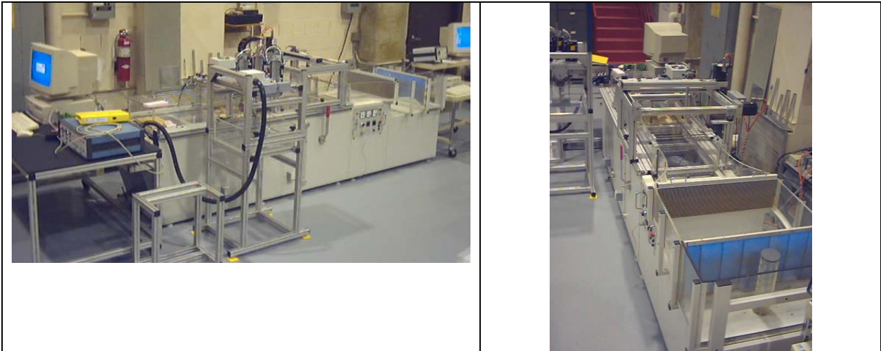
Figure 1. Test flume, trumpet shaped inlet and Multi-Hazard Lab
