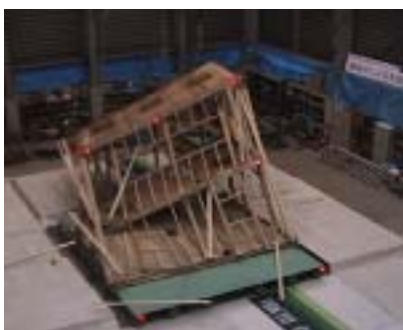
Fig. 12 Preliminary 3-D Shaking Table Test
