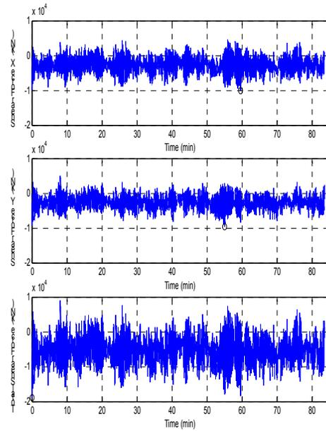
Figure 1. Base shear forces in the  $x$  direction (top), in the  $y$  direction (middle) and the total shear (algebraic sum).
