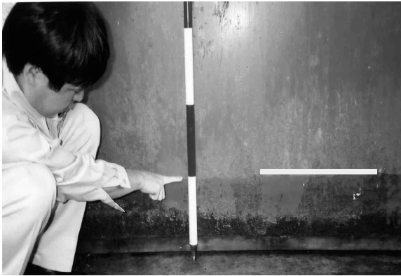
Picture 7. Tsunami Inundation Sign on the Wall of the Warehouse in the East Port of the Kushiro Port
