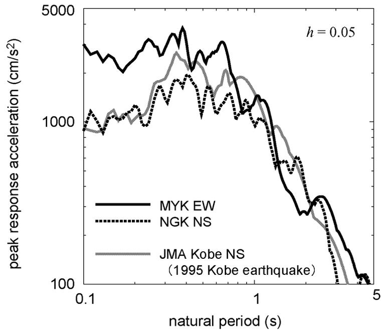
Fig. 4: Response spectra (damping ratio of 5%)
