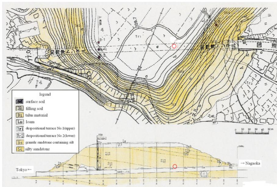
Fig. 18: Plan view and longitudinal section of Wanatsu Tunnel with geological formation
