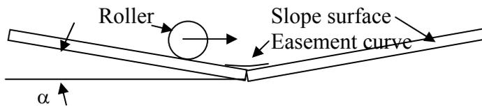
Figure 1. Conceptual assembly of bearing
