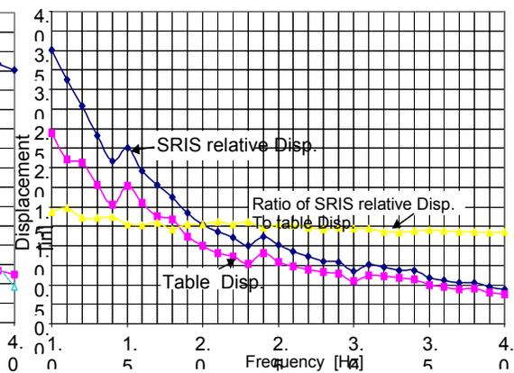
Figure 3. Displacement under sweep sine test
