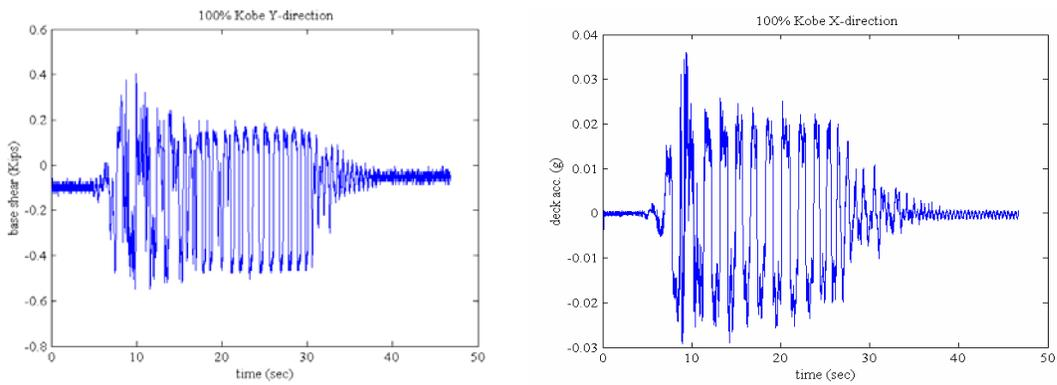
Figure 5. Base shears under earthquake excitation
