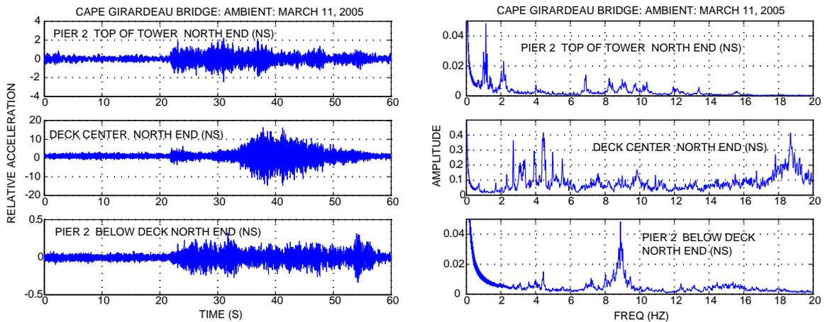
Figure 6. Sample ambient vibration response (recorded in real-time and on demand) and corresponding amplitude spectra at three bridge locations.
