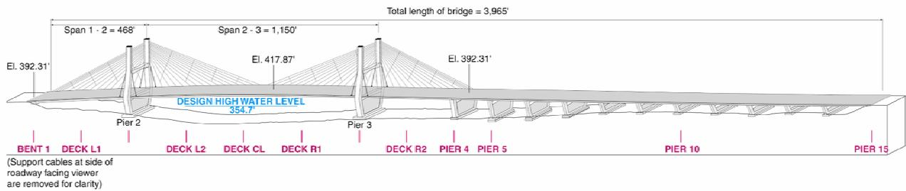
Figure 2. General schematic and dimensions of Bill Emerson Memorial (Cape Girardeau) Bridge.
