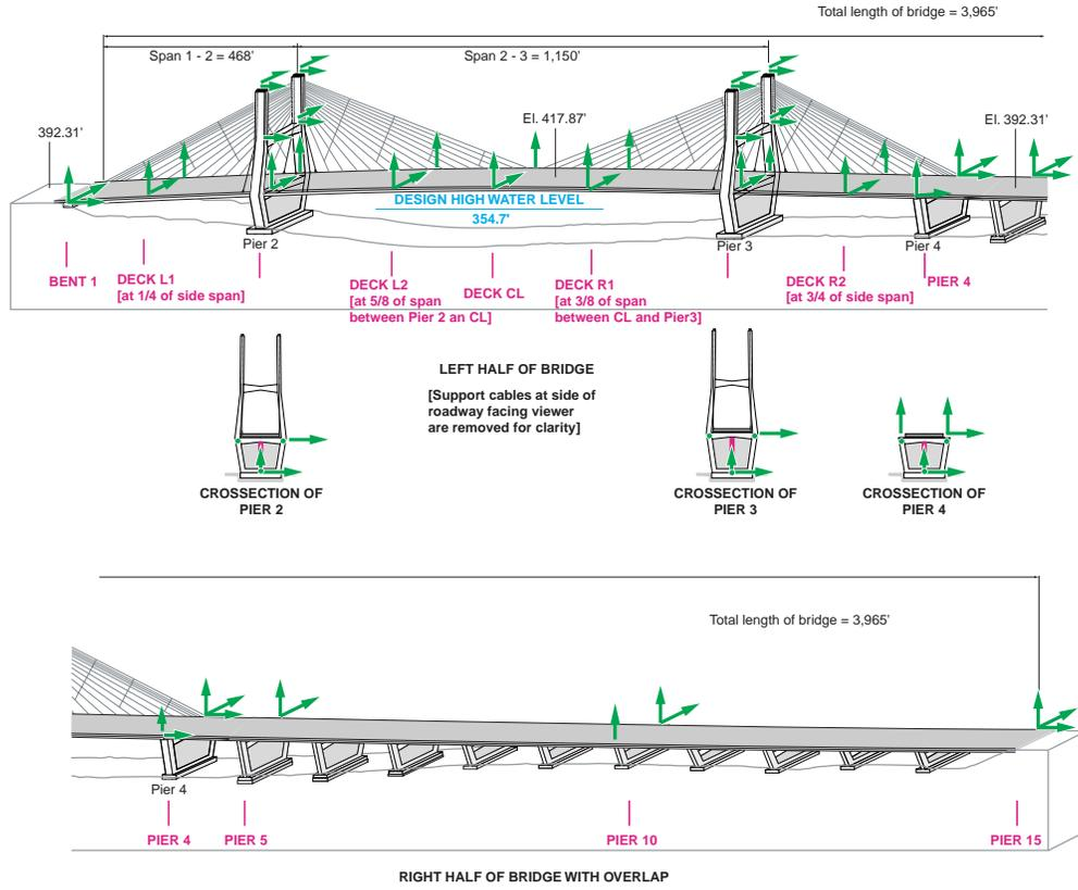
Figure 5. Enlarged three-dimensional view of the Bill Emerson Memorial (Cape Girardeau) Bridge, significant locations identified for seismic instrumentation and distribution and orientation of the accelerometers.
