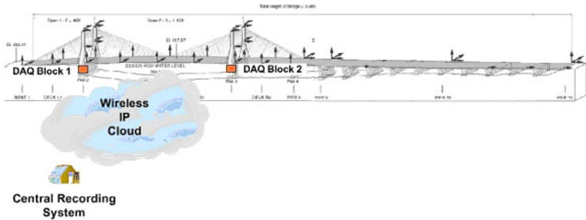
Figure 3. General Schematic of the seismic monitoring system using Data Acquisition Blocks 1 and 2 at the Piers 1 and 2, off-structure Central Recording System and wireless communication technology (Wireless IP Cloud).
