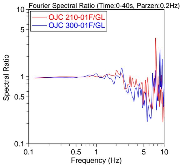
Fig. 6 Fourier spectral ratios, 01F/GL, in horizontal directions at OJC
