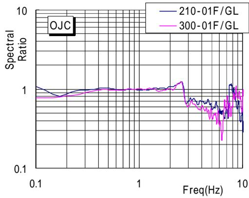
Fig. 11 Fourier spectral ratios 01F/GL in horizontal directions about OJC
