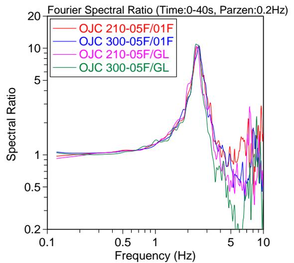
Fig. 7 Fourier spectral ratios about Top/Base and Top/GL at OJC
