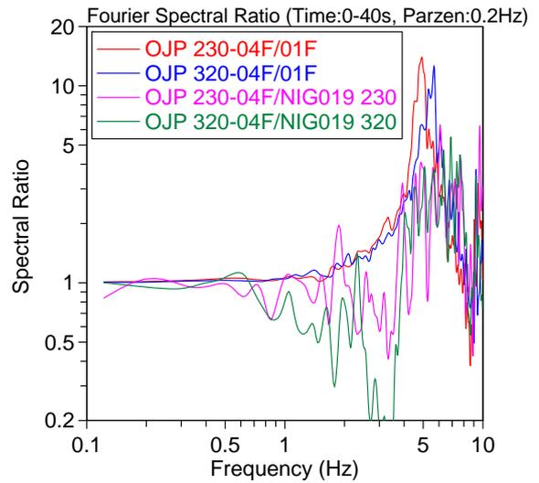
Fig. 10 Fourier spectral ratios about Top/Base and Top/GL at OJP
