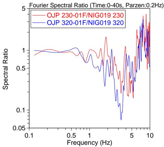
Fig. 9 Fourier spectral ratios, 01F/GL, in horizontal directions at OJC
