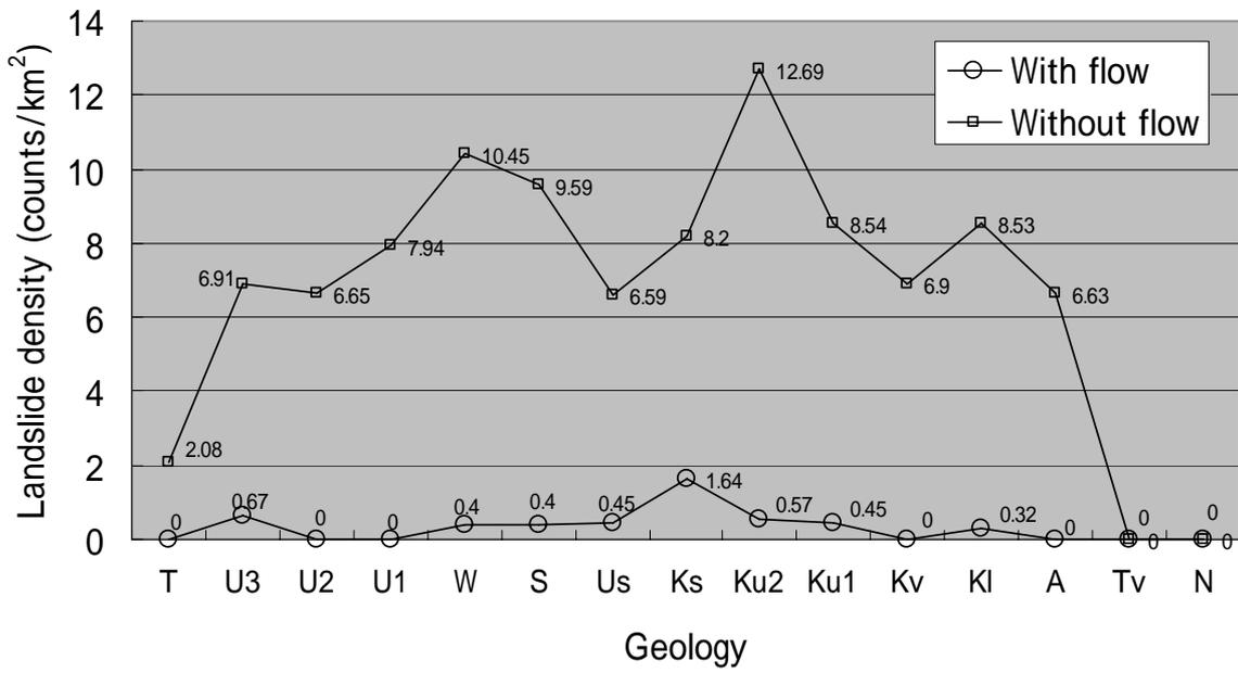
Fig. 6 Landslide density in each geological formation, correspondent to Table 1 and Fig. 5.
