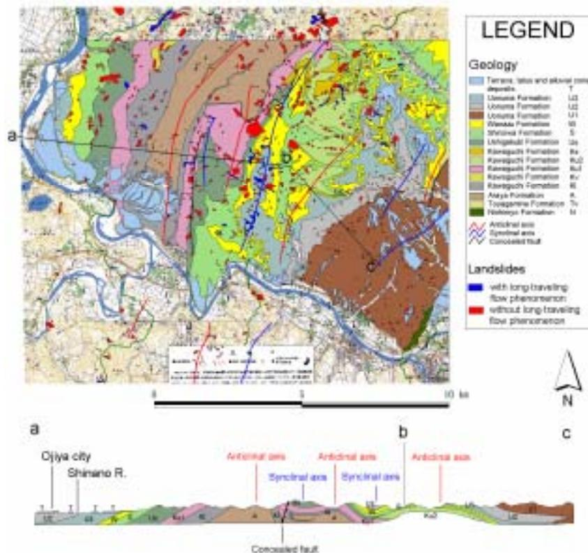
Fig. 5 Overlay of landslide distribution over the geological map. The geological map and cross section of the geology are a part of [7].
