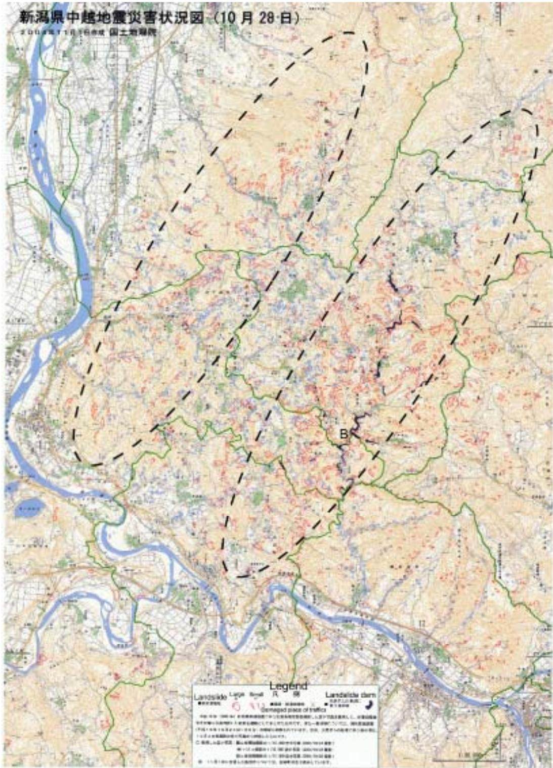
Fig. 2 Distribution of landslides triggered by the earthquake. Mapped landslide dams indicate the areas as of October 28, 2004. Black dotted lines and site “B” were added on the original “Disaster Map” (Geographical Survey Institute [10]).
