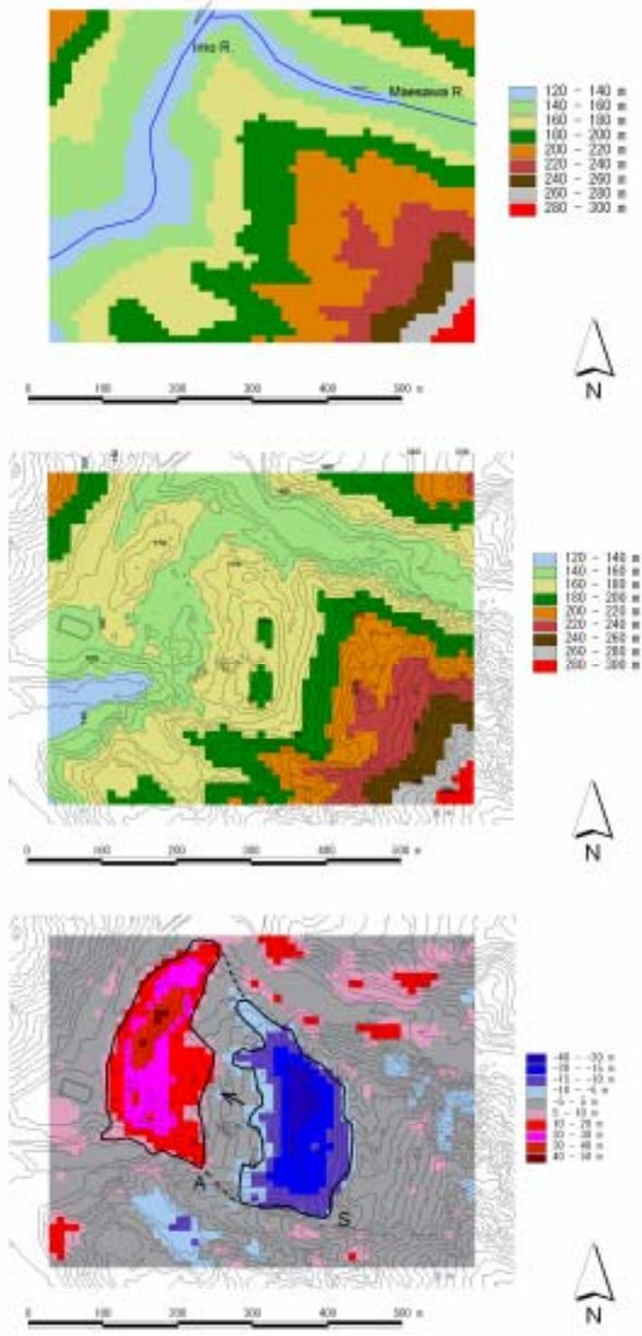
Fig. 3 Topography change between pre- and post-earthquake. The pre-earthquake DEM (upper) was derived from 1:25:000 contour map. In the middle figure, the post-earthquake DEM is superimposed on the contour lines, which were derived from the airborne LIDAR data, are in meters.
