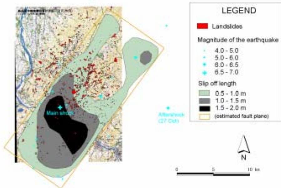
Fig. 4 Overlay of landslides distribution on the seismicological data (magnitude data, [1]; calculated fault plane and slip off length, [3]).
