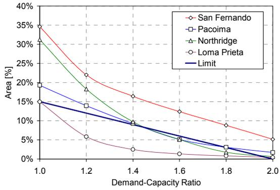
Figure 10. Comparison of percentage of overstressed areas with acceptance limits
