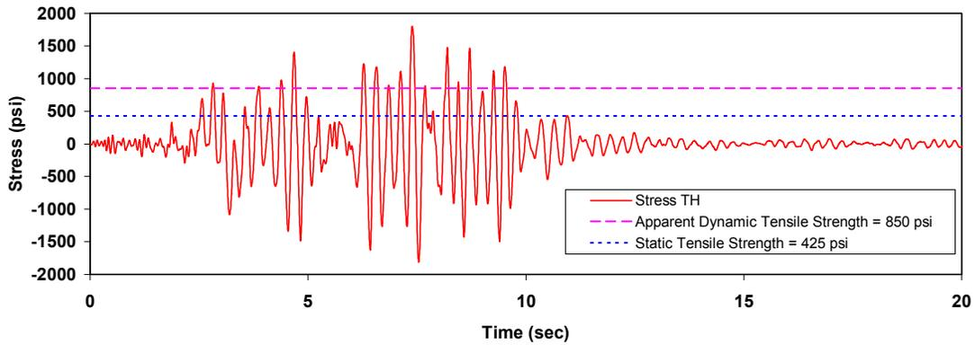
Figure 8. Time history of maximum vertical stresses at the heel of the dam for San Fernando record.
