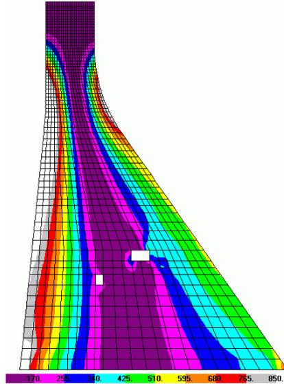
Figure 7. Envelopes of maximum vertical stresses for San Fernando record (linear model)
