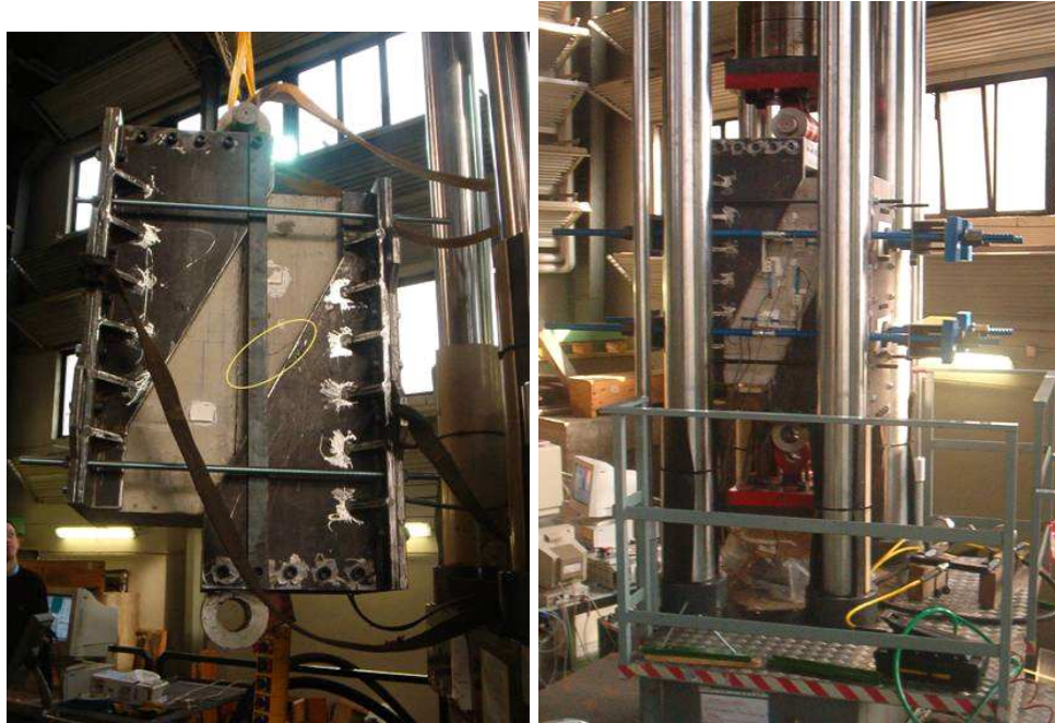
Figure 4: Large Scale Testing of Concrete Joints Subjected to Reverse Cyclic Loading
