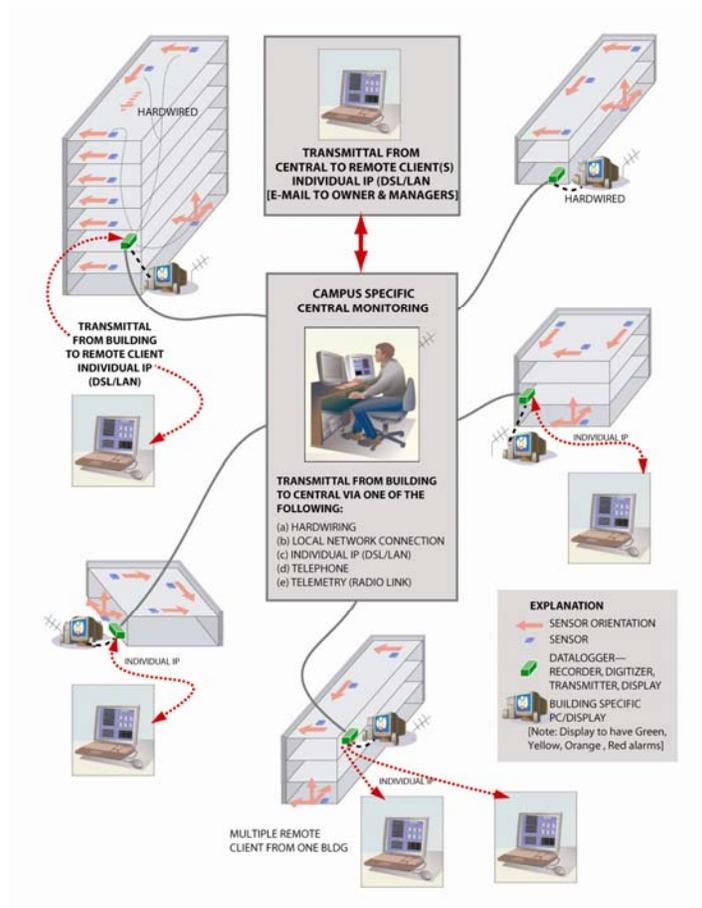
Figure 8. A schematic of campus oriented monitoring system. Each building within a campus may have its own monitoring system or there may be a central monitoring unit.
