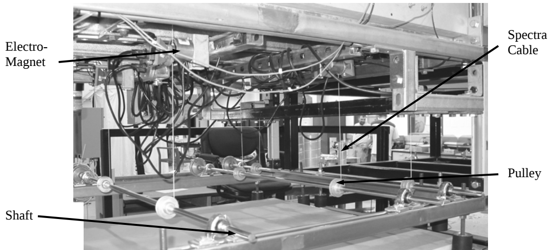
Figure 3: Free-vibration suspension system initial condition apparatus.
