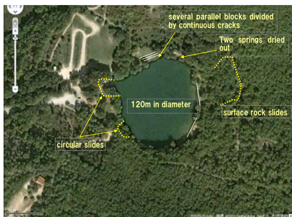
Photo 3 Lateral spreading around Lake Sinizzo (added on Google map)
