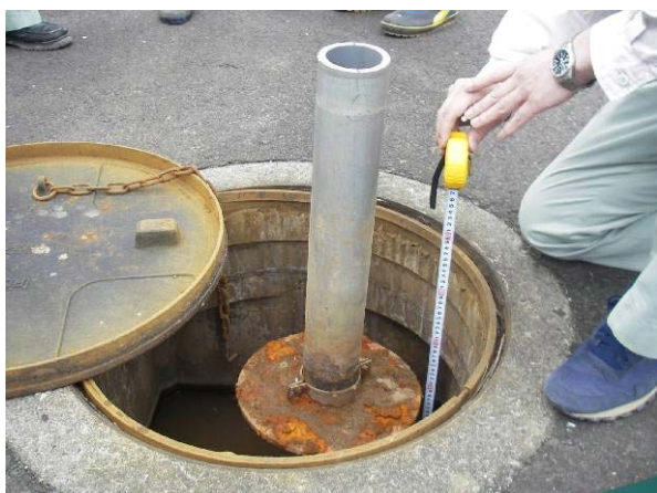
Photo.8 The pipe of a crossarm gauge protruded, as a result of the settlement of the dam body (Aratozawa Dam) (Photographed by PWRI on June 16, 2008)
