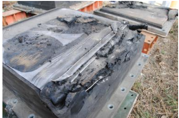
Photo 12 One of elastomeric bearings ruptured
