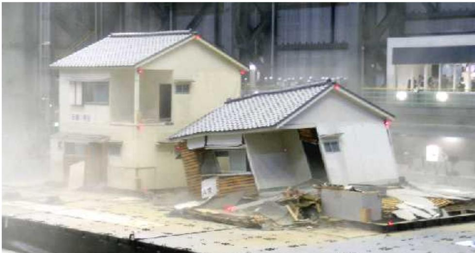
Photo 2. Shake Table Test by E-Defense (Left: Retrofitted, Right: ‘As-built’)
