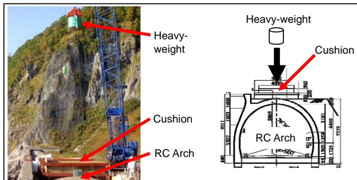
Fig.1: Heavy-weight-falling Experiment for RC Arch
