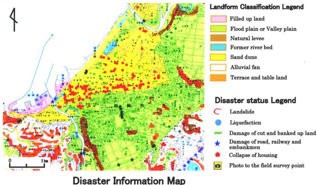
GSI performed post disaster investigations of the damage caused by landslides and liquefaction, to roads and railways, collapse of houses as well as their distribution and scales, which were compiled into a Disaster Status Map. The Map was made available to the public on GSI's Web Site.
