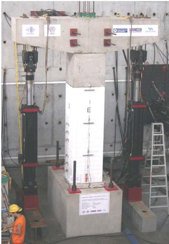
**Precast Segmental Column Prior to Seismic Testing**
