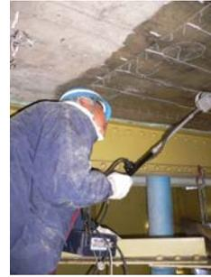
NDE for deterioration of deck plate
