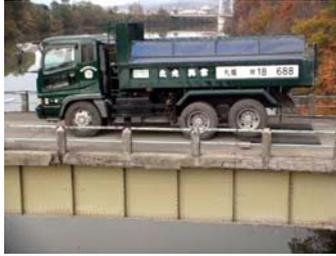
Truck load test for vehicular breaking forces
