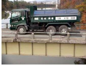
Truck load test for vehicular breaking forces
