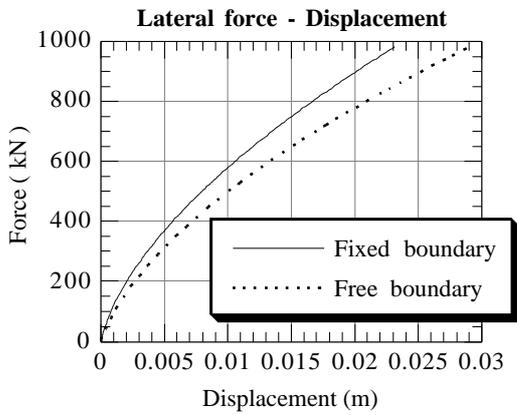
Figure 7 Lateral force - displacement relationship with 3D FEM analysis
