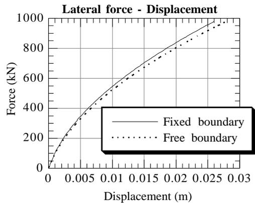
Figure 3. Lateral force - displacement relationship with MRO model
