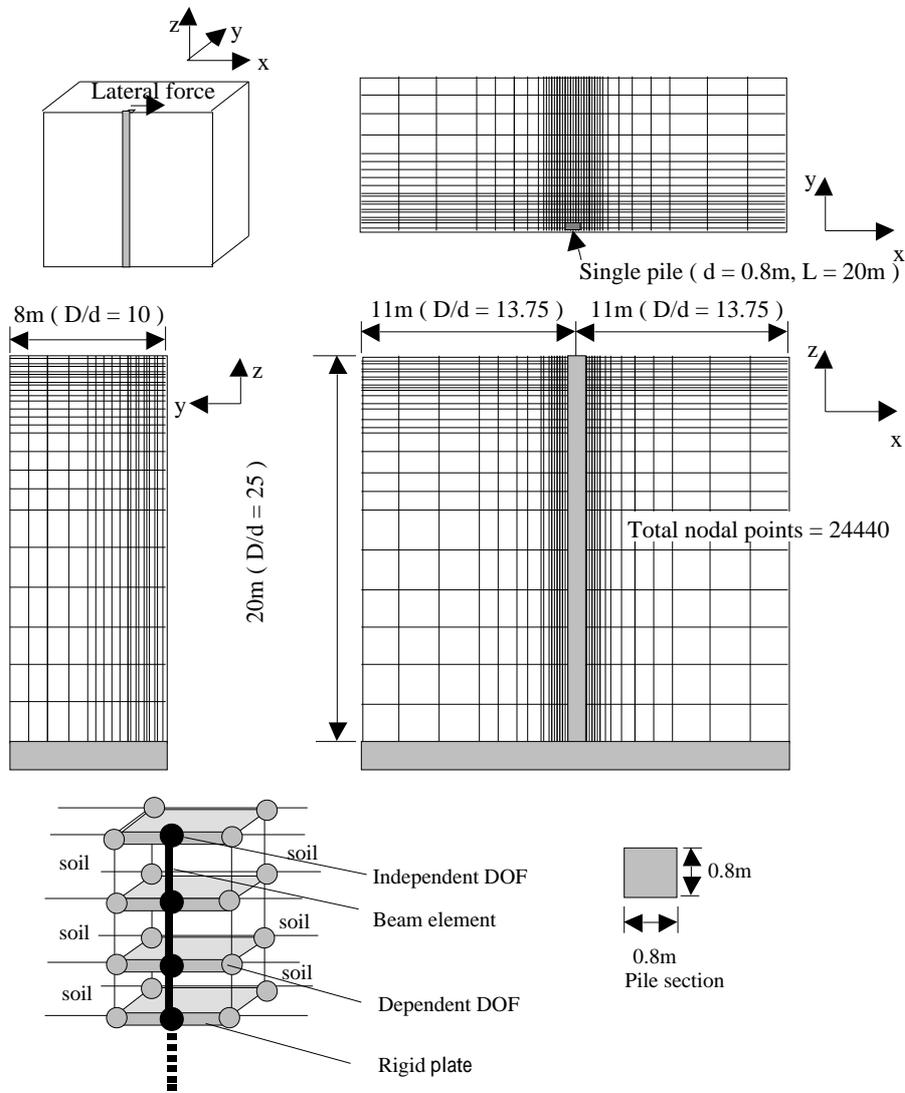
Detail of a single pile model considering its volume
