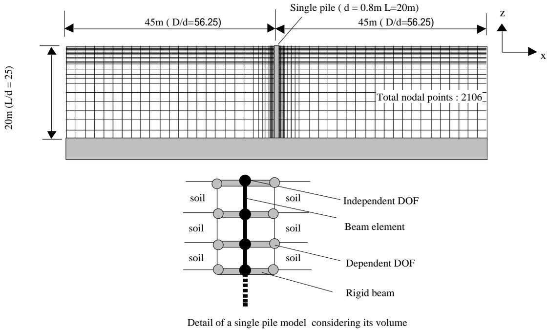
Figure.1 2D FEM model for a single pile - soil interaction analysis.
