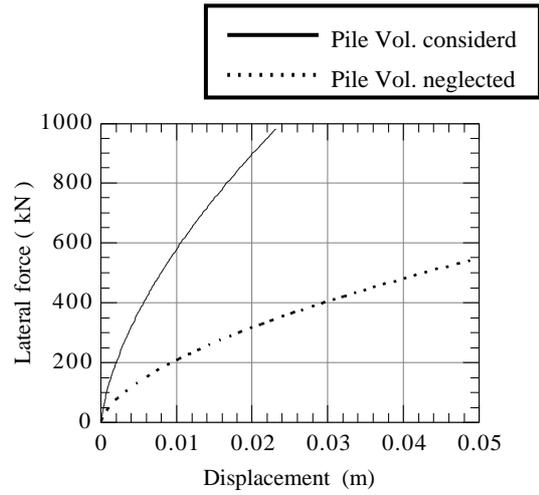
Figure 9 Lateral force - displacement relationship with and without pile volume considered.
