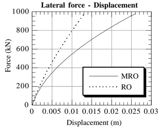
Figure 5. Comparison of lateral force - displacement relationship with MRO and RO model.
