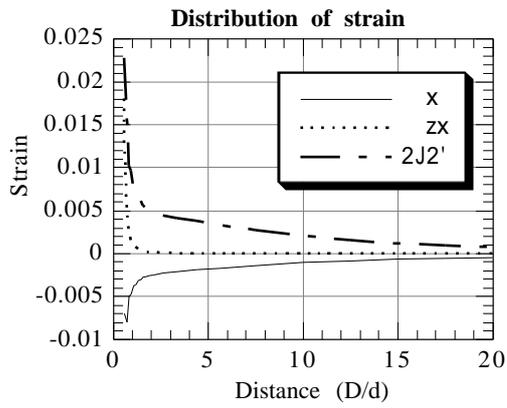
Figure 4. distribution of maximum strain along soil surface at GL-10cm.
