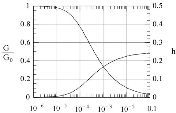
Figure 2 Strain dependency of stiffness and damping expressed by MRO model.
