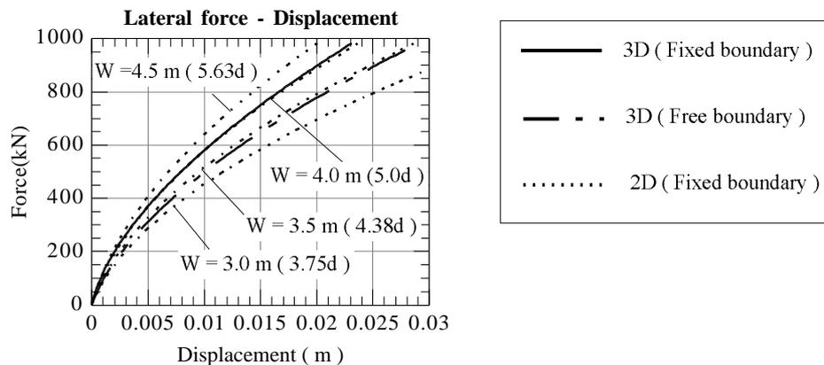
Figure 9 Comparison of 2D and 3D FEM analysis.
